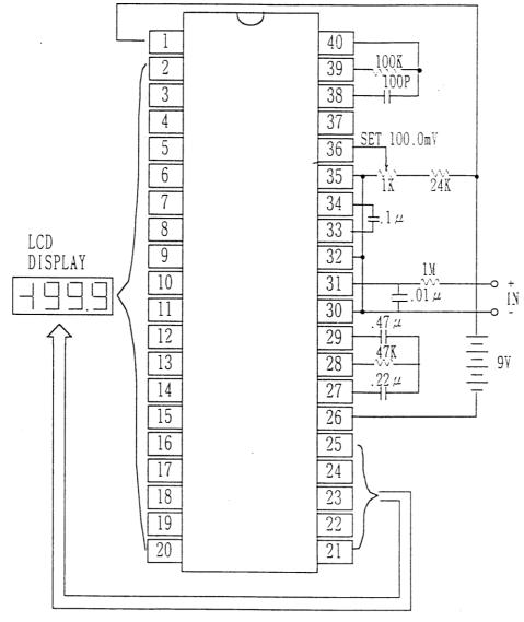
Clock Frequency 48 KHz (3 readings/sec)
