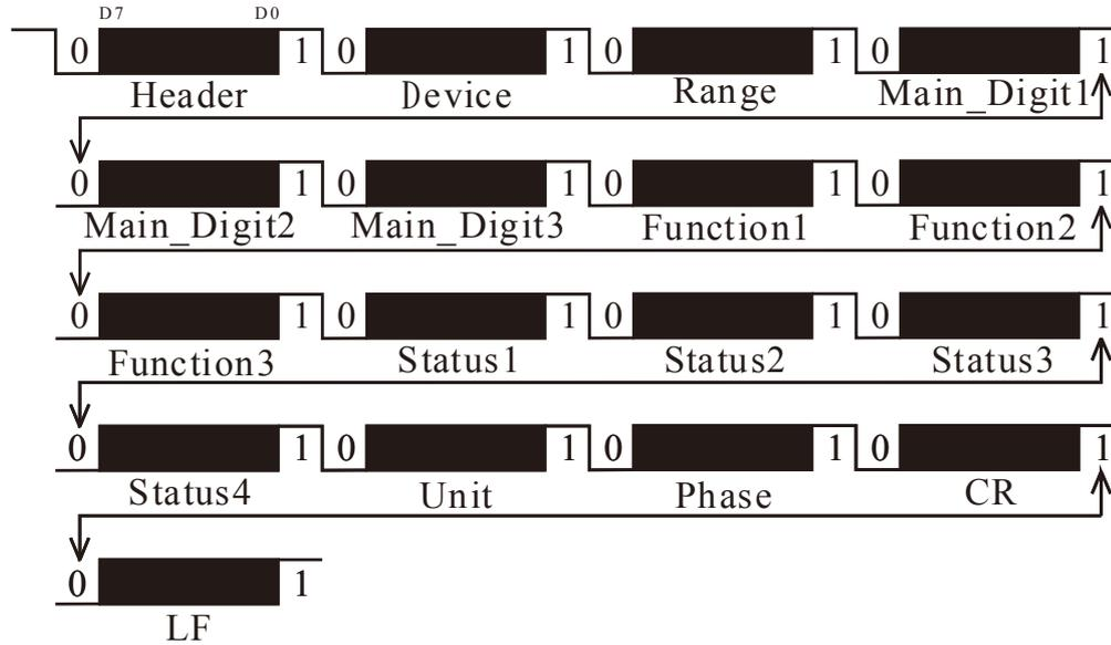
The meter always outputs the current value shown on LCD screen to the serial port. The detailed data format of each packet is listed below.
