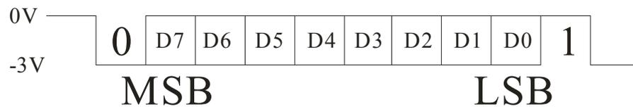
One data block consists of 17 packets. The following figure shows the format of a data block. The Header and Device code leads the whole packets. The range packet indicates the decimal point position on LCD panel of meter. Main\_Digit1-3 consists of the readings on the LCD panel. The function packet indicates the measurement mode of the meter. Status1-4, Unit, Phase give the other status of the meter. CR and LF are delimiters used to separate the blocks.
