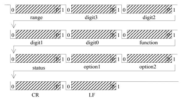
The meter always outputs the current input value to the serial port in spite of HOLD mode. Each block is repeated twice in one conversion cycle. The detailed data format of each packet is listed below.
