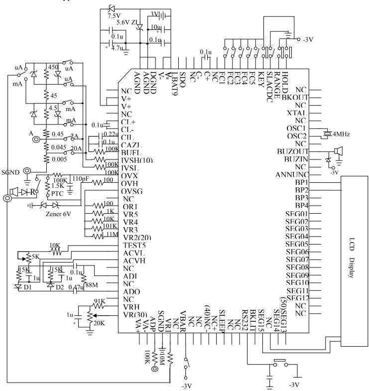
Note: In order to prevent IC from damaging by inappropriate operation, the Zener diodes **MUST** be required as protection.
