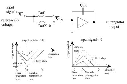
Figure 1. the structure of dual-slope integrator and its output waveform.
