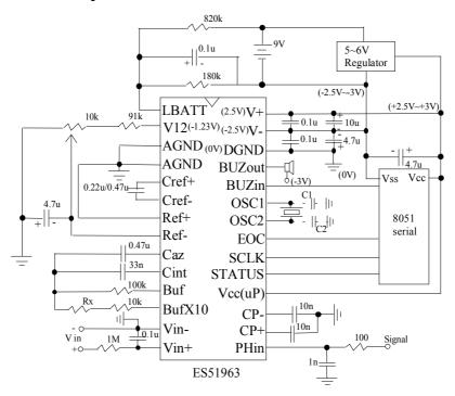
9V battery and 3.3V/3.0V microprocessor:
