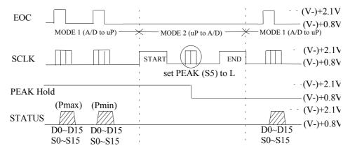
Note: After changing X10 mode at format 1 or format 2, if we want to active PEAK Hold function, we must active calibration again.
