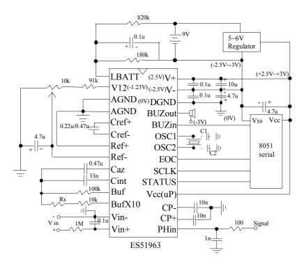
Note: 1. Vin+, Vin- are differential inputs.
