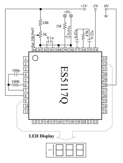
Clock Frequency 48KHz (3 readings/second)
