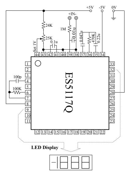
Clock Frequency 48KHz (3 readings/second)
