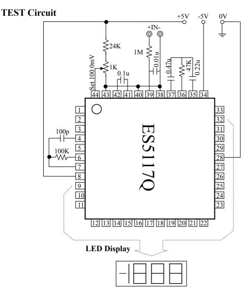
Clock Frequency 48KHz (3 readings/second)
