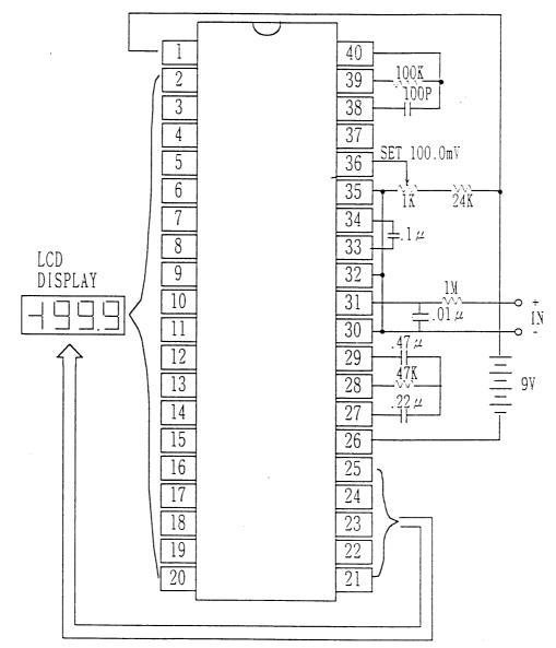
Clock Frequency 48 KHz (3 readings/sec)
