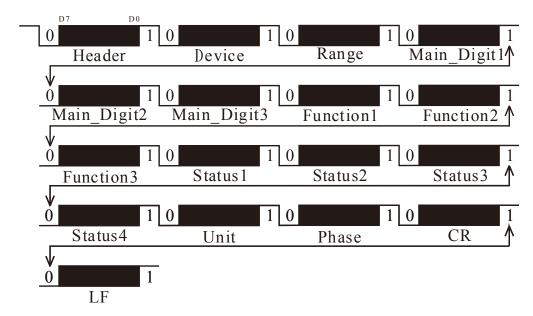
The meter always outputs the current value shown on LCD screen to the serial port. The detailed data format of each packet is listed below.
