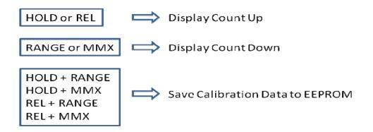
The semi-auto calibration scheme supports the following eleven measurement modes. When *CALEN* pin is active, set the proper function switches or push KEY to choose the target measurement mode. When mode is selected, the LCD segment of Unit at related measurement will be blinking.
