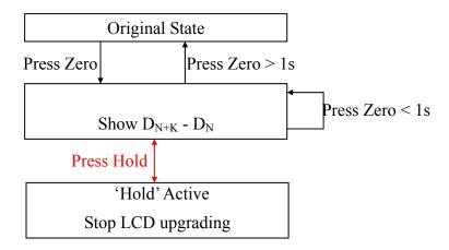
• State diagram for ZERO + Max/Min + HOLD mode :
