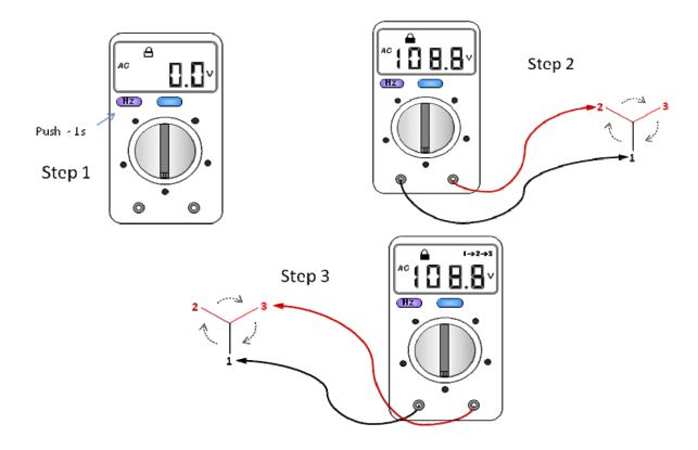
Note: The time limit is 5 seconds between Step2 & Step 3.
